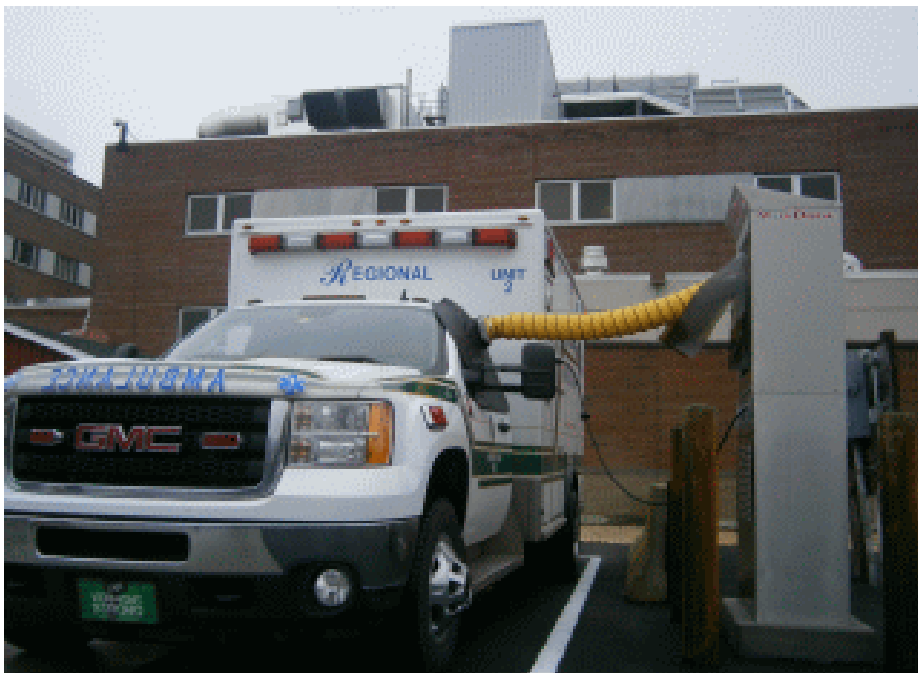
Figure 2: Ambulance connected to MediDock EPS Kiosk (HVAC and power). Courtesy of Vermont Department of Environmental Conservation.
